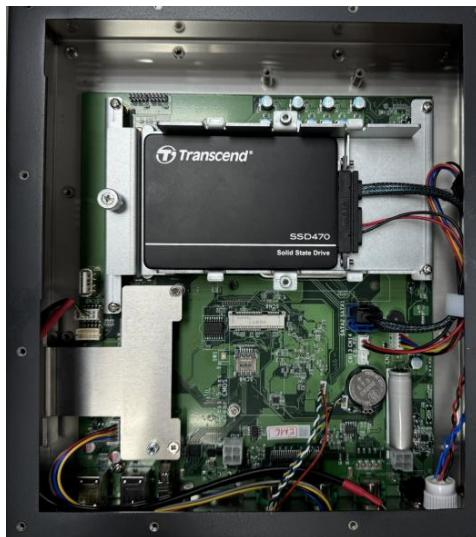
Step 8 The IPC980 supports an optional second HDD/SSD. Fix HDD/SSD to the HDD bracket with four screws.
