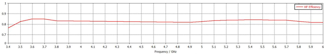
\*Efficiency simulated in CST Microwave Studio excluding cable loss.
