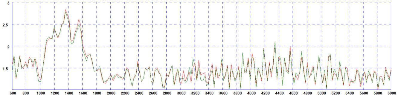
\*VSWR for elements assemblies 1 and 2 measured with 5m (16') of CS32 cable.
