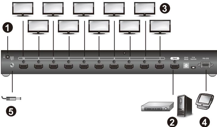
1. Use a grounding wire to ground the unit by connecting one end of the wire to the grounding terminal, and the other to a suitable grounded object.
