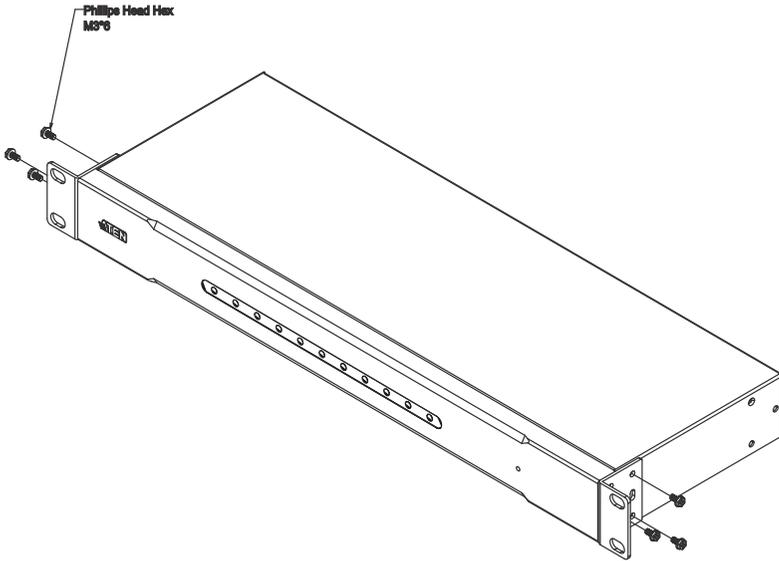
2. Screw the mounting brackets to the rack.
