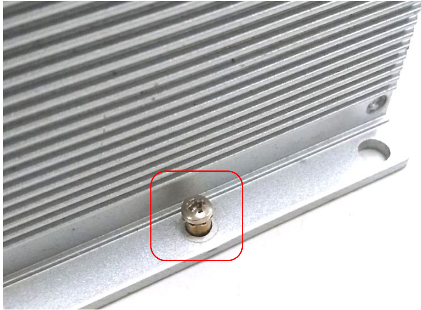
Ground screw of router
