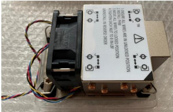
This cooler is for CPU above 205 Watts.
