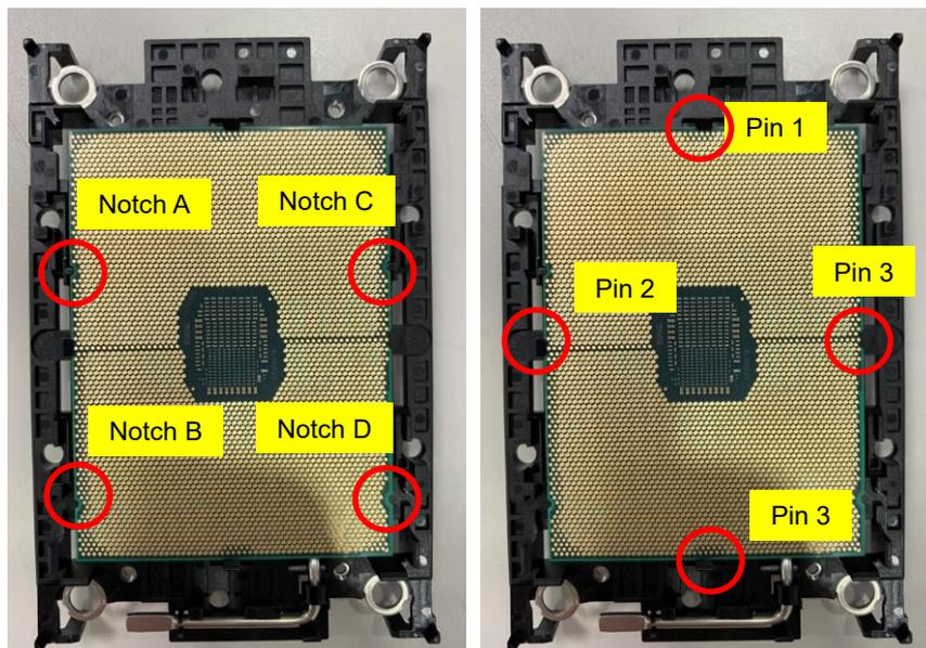
**Step 3** Check the notch on the CPU and the pin on the CPU socket of IMB760.
