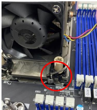
**Step 6** Use a T30 Torx screwdriver (8in-LBF) to tighten the screws on the cooler.
