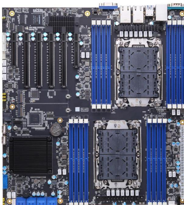
The IMB760 is an advanced EATX industrial serverboard based on the Intel® Xeno® Scalable Ice Lake-SP processors in dual LGA4189 socket, and it comes with an Intel® C627A chipset. Featuring optimal computing and visual performance, the IMB760 motherboard is an ideal solution for developing major industry applications ranging from financial modeling to deep learning AI and complex video analytics.
