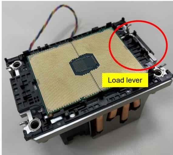
**Step 4** Place the CPU cooler module on the CPU socket on the motherboard, and then align pin A to hole A and pin B to hole B simultaneously.
