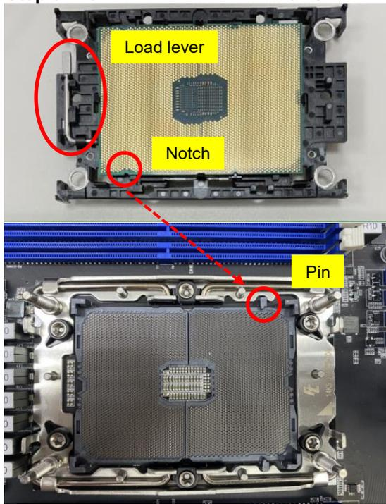
Follow the installation direction and Install the CPU clip and CPU on the cooler module.
