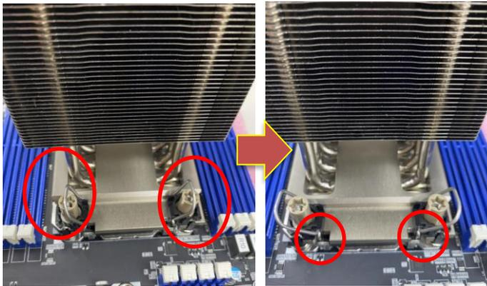
**Step5** Put the fan module on the CPU cooler and tighten two screws (8in-LBF).
