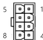
ATX2 ATX 12V power input connector:
