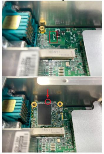
Step 4 Tighten the screw tightly.
