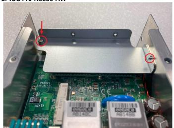
Step 7 Put the cover back to the system and tighten the screws then close the chassis.
