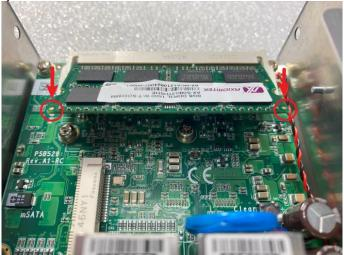
Step 4 The memory module is locked by two latches on the sides. We strongly recommend using "LDC737" silicone on both sides of the memory for better anti-vibration.
