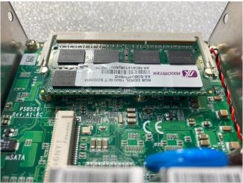
Step 5 Put the thermal pad on the memory module to improve the cooling effect. For ICO110-N3350-AW
