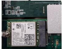
Step 2: Unscrew the 4 screws on the back maintenance window cover and remove the antenna plug from one of the antenna holes on the system chassis.
