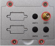
Step 4: Connect the other end of the cable to the connector on the wireless module.
