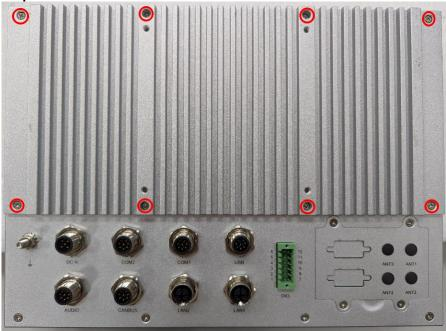
Step 2 Open the back heatsink and locate the M.2 and Mini card slot on main board.
