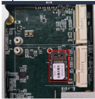
Step 3: Close the top cover and pushit down to secure the SIM Card.
