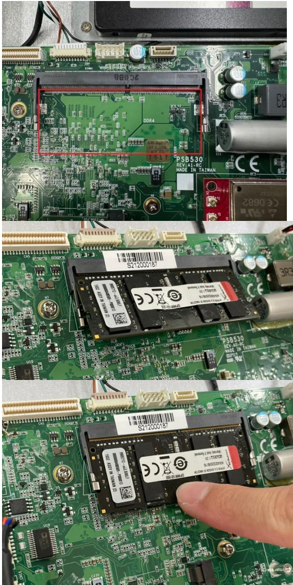
Figure 2-14: Installing a memory module
