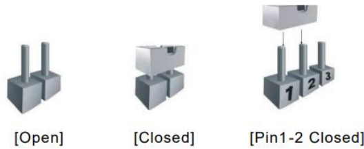
Figure 2-3: Definitions of pin settings
