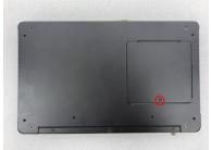
Step 3 Open the DRAM cover and locate the SO-DIMM socket on the board.
