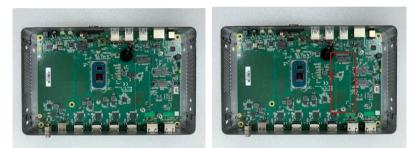
Step 4 Identify the M.2 M Key slot, insert a SSD module into the socket and then fasten a screw.
