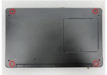
Step 3 Open the TOP cover , located the M.2 socket on main board.
