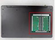
Step 4 Insert a gold-colored contact into the socket and push the module two end latches till locked of the DRAM.
