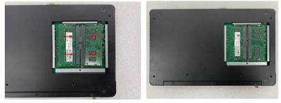
Step 5 Put the DRAM cover and fasten one screw back into the system.
