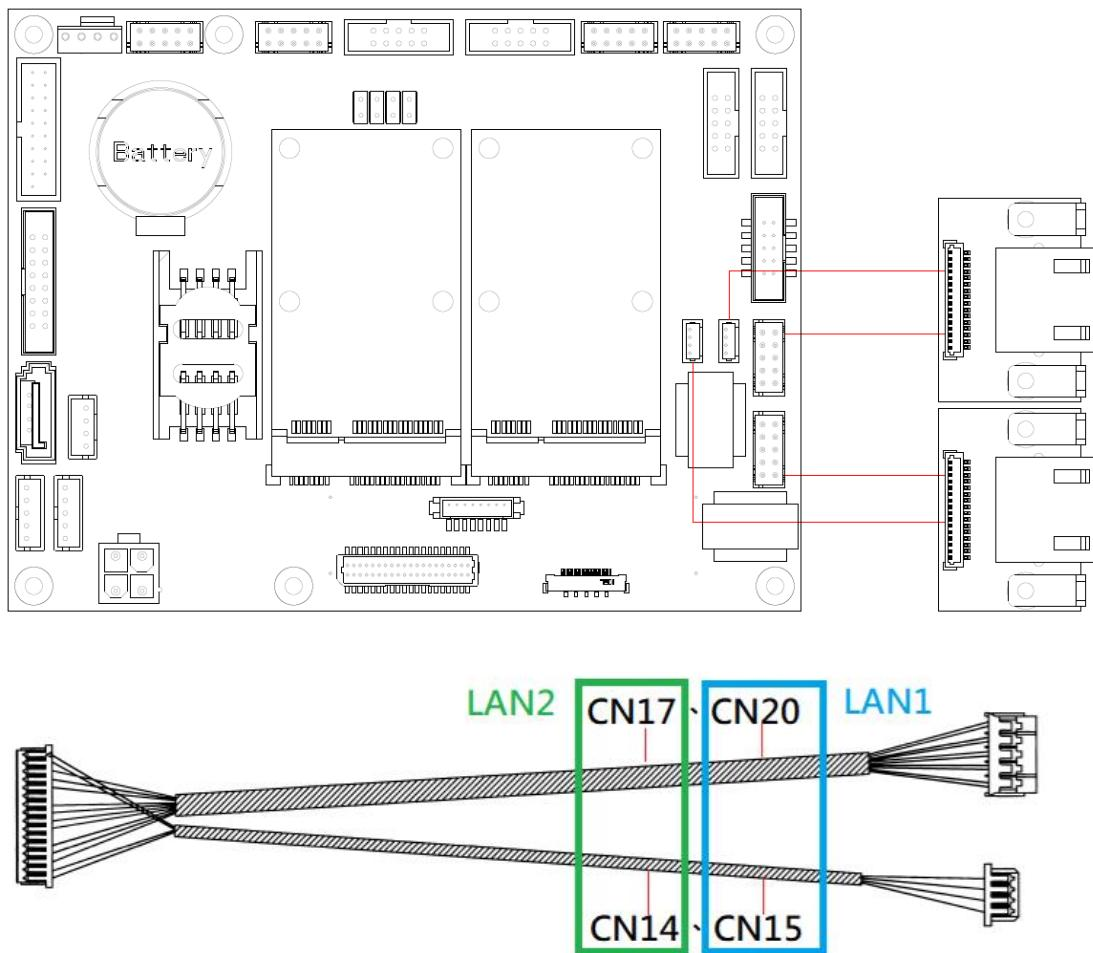
\*There are total 2 x GbE, LAN1 & LAN2, from CEB94021, and please make sure LAN cable (59440212700E) is assembly to corresponding box wafer that shows above.
