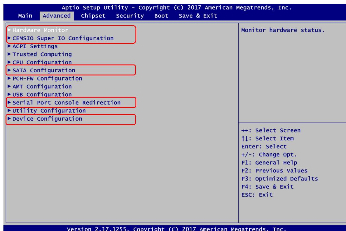
The sub menus marked with red rectangular contain functions available only if CEB94021 is connected to CPU module. The functions are COM port settings in Super IO Configuration, digital I/O settings in DIO Configuration, Serial Port Console Redirection and an extra mSATA/PCIe selection in SATA Configuration.
