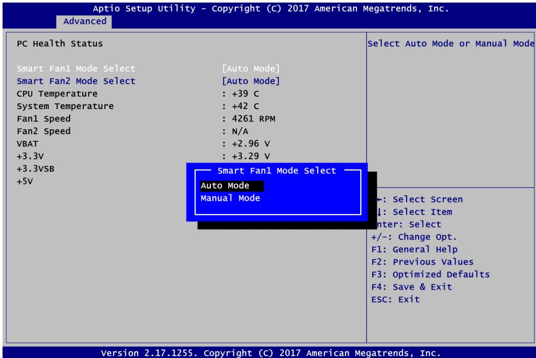
This screen displays the temperature of system and CPU, cooling fans speed in RPM and system voltages (VBAT, +3.3V, +3.3V standby and +5V).
