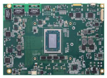
The CAPA13S, a 3.5" board, supports AMD® RYZEN® Embedded V1605B/V1807B processor. It delivers outstanding system performance through high-bandwidth interfaces, multiple I/O functions for interactive applications and various embedded computing solutions.
