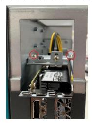
**Step 10** Close the cover back to the chassis and fasten the screw. The installation is complete.
