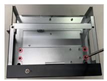
**Step 6** Screw the fan module into chassis and plug in the fan connectors.
