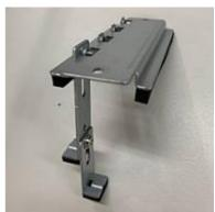
**Step 9** Fasten the holder bracket in the chassis, adjust the screw position of the extension bracket to fix the add-on card, and then screw it.
