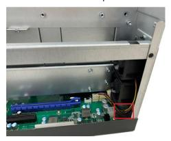
Step 8 Remove the slot brackets.
