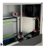
Step 12 Paste the Mylar on the vents of the system cover.
