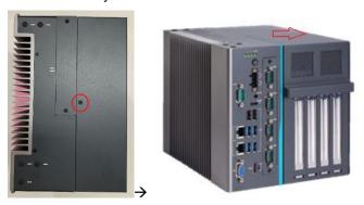
**Step 5** Unscrew the bracket, fasten the fan module into the expansion box and plug cable(s) to connector(s).
