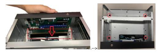
**Step 6** After installing the expansion box kit, close the system cover back to the chassis and fasten the screw. Installation is complete.
