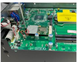
**Step 6** Remove the antenna plugs from the top of back cover, and then install the antennas on the antenna connectors.
