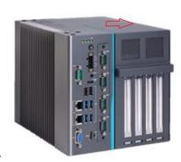
Step 5 Unscrew the bracket, fasten the fan module into the expansion box and plug cable(s) to connector(s).
