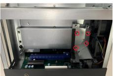
**Step 10** Align the A2 card with the slot, press the card into the slot until it is firmly seated, and screw the A2 card bracket and slot bracket to the chassis.
