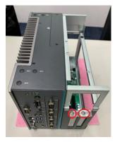
**Step 9** Insert the air duct bracket's metal part as marked A below and screw the 4 screws.
