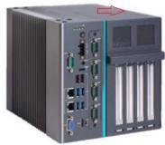
**Step 4** Locate the PCI or PCIe slots and remove the slot bracket from the slot in which you want to add the card.
