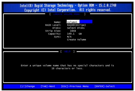
3.4. When finished, press <Enter> to select a RAID level. There are two RAID levels: RAID0, RAID1. Select a RAID level and press <Enter>.
