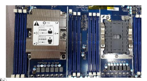
Note: To protect the CPU socket pins,do not remove the CPU cap when the CPU is not installed.
