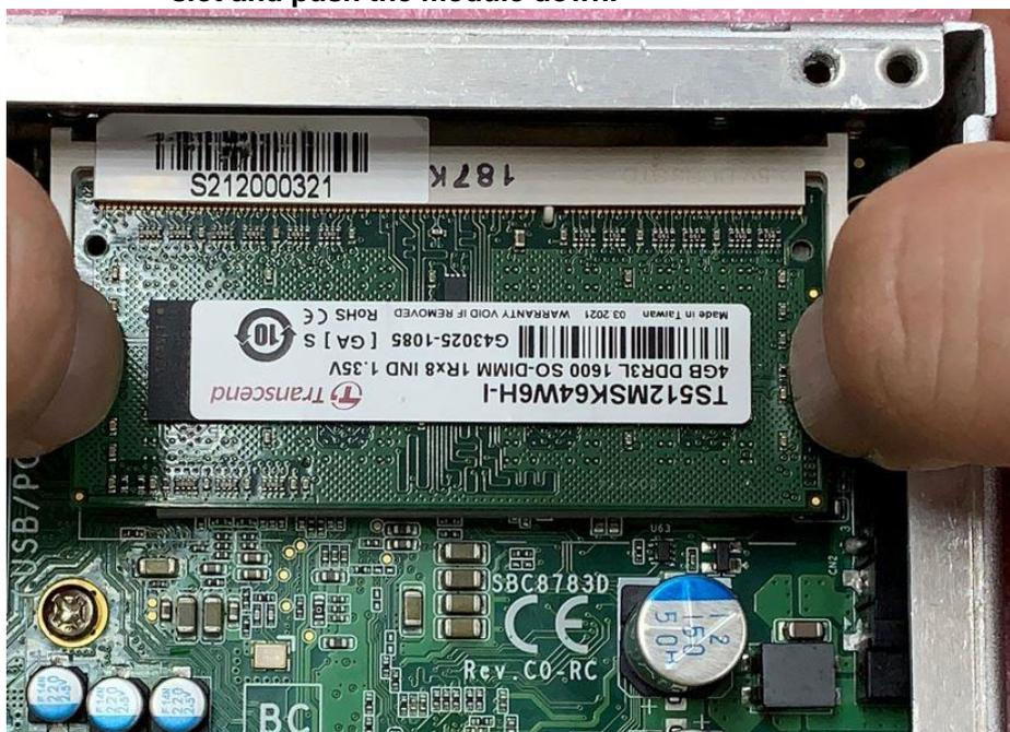
**Step 5** The memory module is locked by two latches on the sides. We strongly recommend using “LDC737” silicone on both sides of the memory for better anti-vibration.
