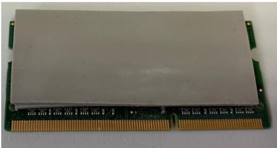
**Step 4** Use two fingers to hold the memory module and insert the gold figure into the slot and push the module down.
