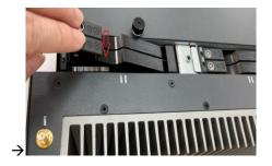
**Step 6** Screw the bracket. The installation is complete.
