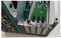
**Step 2** Align the PCI or PCIe card with the slot, press the card into the slot until it is firmly seated and screw it.
