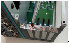
**Step 2** Plug two graphics card power cables in AX98268. (Please refer to the note of maximum power loading limitation.)
