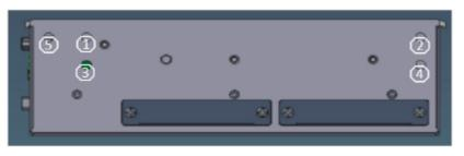
Step 7 Close the heatsink cover to the chassis and fasten all screws. The installation is complete.
