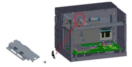
Step 7 IPC962A and IPC964A offer 3 types of extension holder brackets. Please take the brackets and screws from the accessory box and assemble the extension holder bracket. The procedure is illustrated below.
