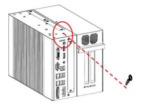
Step 5 Insert the SSD card to slot and push it down firmly. Then fasten the card tightly to the mainboard.
