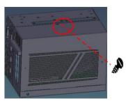
Step 4 Loosen the screw to remove the bracket.
