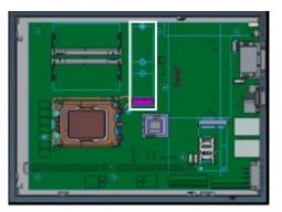
Step 6 Paste the other thermal pad on the module and then remove the protective film.
