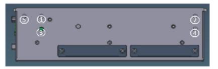
Step 8 Close the heatsink cover to the chassis and fasten all screws. The installation is complete.
