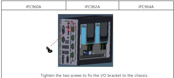
Step 7 Screw the extension I/O bracket into system as shown below.
