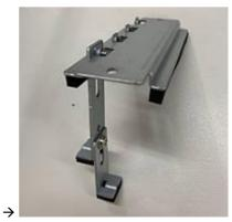
Step 9 Fasten the holder bracket in the chassis, adjust the screw position of the extension bracket to fix the add-on card, and then screw it.
