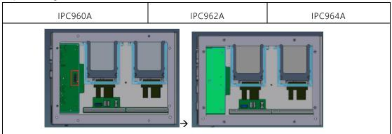
Align the I/O module with the slot, press the module into the slot until it is firmly seated..
