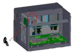
Step 10 Close the cover back to the chassis and tighten the screw. The installation is complete.
