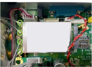
Note: The 5G, LTE and Wi-Fi modules come with a different type of SMA cable, one is IPEX, and another one is IPEX4. Please do not mix them up to avoid mismatch.
