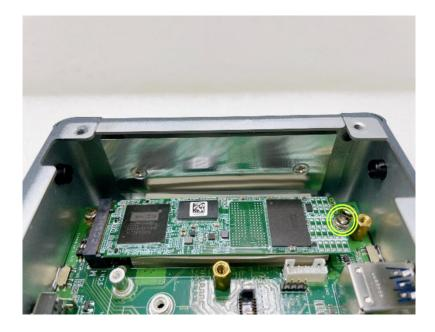
Step 9 Place the SSD thermal bracket on the M.2 2280 Key M SSD drive, then secure the bracket to the carrier by firmly tightening the two M3 screws to the marked positions. Ensure that the thermal pad on the side is securely attached to the chassis.
