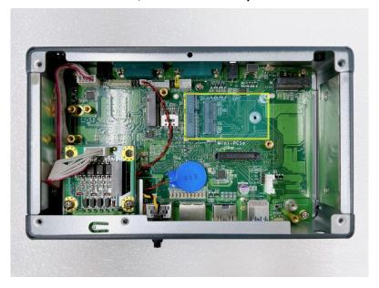
Step 4 Holding the PCI Express mini card at a 45 degree angle up from horizontal, slowly insert the golden fingers into the PCI Express slot until it is fully inserted in.
