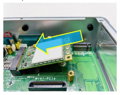
Step 5 Press it down gently, but firmly, and then secure the PCI Express mini card to the carrier by tightening up the one M2 Phillips screw to the marked position.
