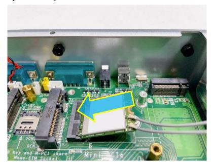
Step 6 Press the M.2 Key E 2230 module down gently, but firmly, and then secure the module to the carrier by tightening up one M3 screw to the marked position.
