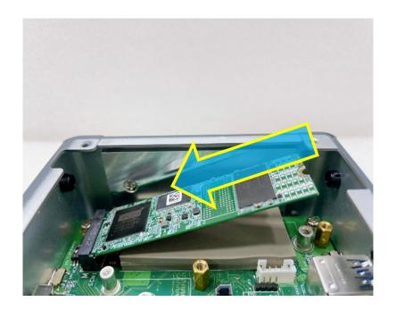
Step 8 Press the M.2 2280 Key M SSD drive down gently, but firmly, and then secure the M.2 2280 Key M SSD drive to the carrier by tightening up one M3 screw to the marked position.
