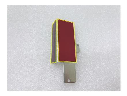
Step 6 Apply two thermal pads onto the M.2 2280 Key M slot.
