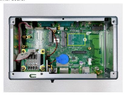
Step 5 While holding the M.2 Key E 2230 module at a 30 degree angle up from the horizontal, slowly insert the golden fingers into the M.2 Key E 2230 slot, until it is fully inserted in place.
