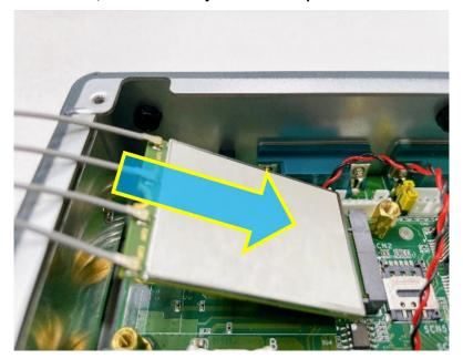
Step 8 Press the M.2 Key B 3052 module down gently, but firmly, and then secure the module to the carrier by tightening up one M3 screw to the marked position.
