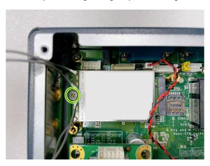
Step 9 Place the 5G thermal bracket on the M.2 Key B 3052 module, then secure the bracket to the carrier by firmly tightening the two M3 screws to the marked positions. Ensure that the thermal pad on the side is securely attached to the chassis.
