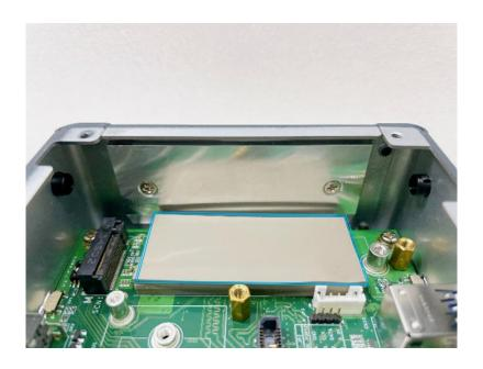
Step 7 While holding the M.2 2280 Key M SSD drive at a 30-degree angle up from the horizontal, slowly insert the golden fingers into the M.2 2280 Key M slot, until it is fully inserted in place.
