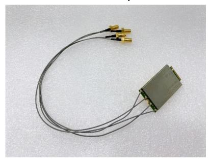
Step 7 While holding the M.2 Key B 3052 module at a 30 degree angle up from the horizontal, slowly insert the golden fingers into the M.2 Key B 3042/3052 slot, until it is fully inserted in place.
