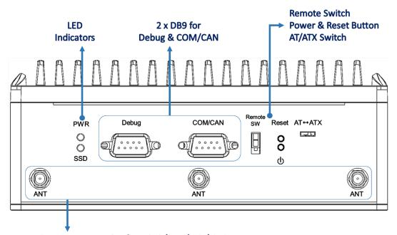
3 x Antenna opening for Wi-Fi / LTE / 5G / GPS Antennas
