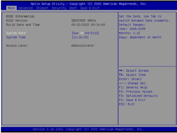
Once you enter the AMI BIOS Aptio Setup Utility, the Main Menu appears on the screen. In the Main Menu, there are several Setup functions and a couple of Exit options for your selection. Use Select Screen Keys (or Move Keys) to select the Setup Page you intend to configure then press <Enter> to accept or enter its sub-menu.
