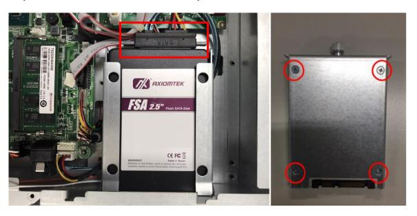
Figure 2-14: Fasten an HDD to the bracket and plug in the "SATA + Power" connector
