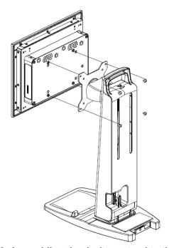
Figure 2-12: Assembling the desktop stand to the panel PC
