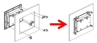
Figure 2-6: Screwing the Panel PC firmly to the panel frame.
