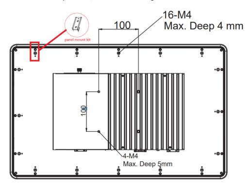
Figure 2-5: Panel mount dimensions (back chassis)
