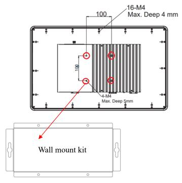
Figure 2-7: Wall mount screwing holes on the back chassis
