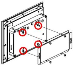
Figure 2-8: Attaching the wall mount bracket
