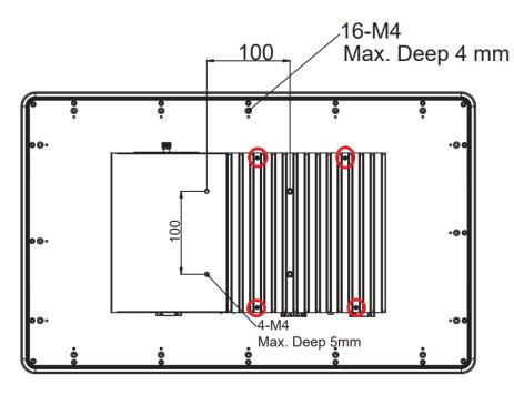
Figure 2-10: VESA mount screwing holes on the back chassis
