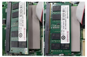
Figure 2-18: Installing a memory module
