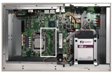
Figure 2-16: DIMM socket position
