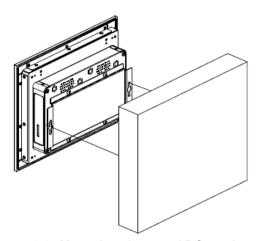
Figure 2-9: Mounting the panel PC on the wall
