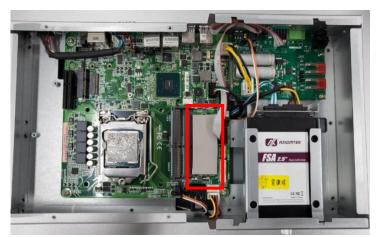
Figure 2-17: Thermal pad position of mainboard
