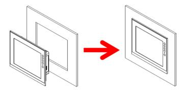
Figure 2-4: Fitting the panel PC into a frame.
