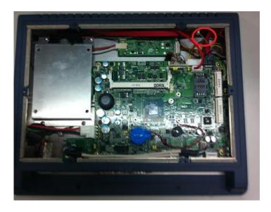
Step 4 There are two connectors on wireless LAN card. One is MAIN, and the other is auxiliary. Connect antenna cable to MAIN connector on wireless LAN card.
