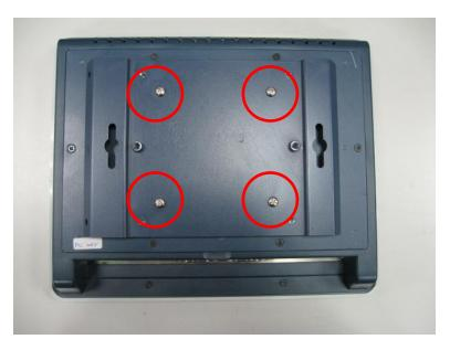
Step 2 Assemble the VESA-ARM to the back side of the chassis, and fix the screws.
