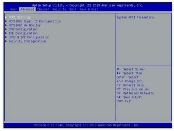
The Advanced menu allows users to set configuration of the CPU and other system devices. You can select any of the items in the left frame of the screen to go to the sub menus:
