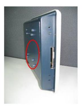
Step 3 Locate the CFast™ socket, and insert the card into the socket.
