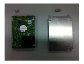
Step 3 Fix the HDD bracket into the system, and plug the data and power cable to HDD. Installation complete.
