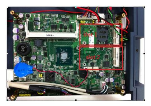
Step 2 Insert the mSATA card to the slot 2. Screw it firmly on the slot.
