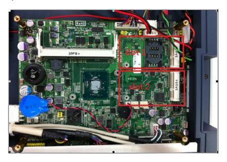
Step 2 Insert the wireless LAN card to the slot. Screw it firmly on the slot.
