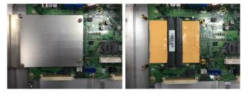
Step 4 Install the DDR module with caution and put the thermal pad on the DDR module again. Than screw the DDR cover to finish the installation.
