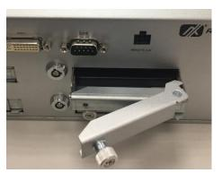
Step 4 Unscrew the rear side screws (x2) and then remove the value-added module slot cover.
