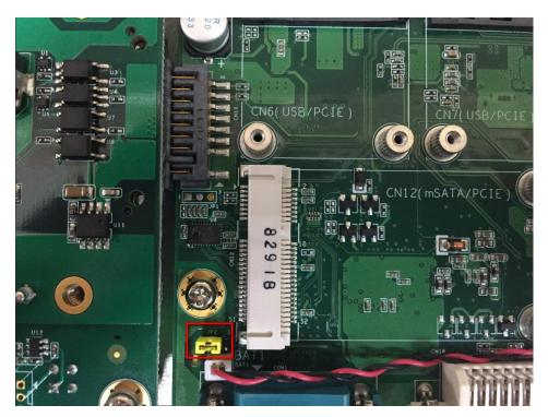
This figure marks the location of the JP2 jumper on the motherboard.
