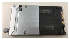
Step 3 Install the SATA drive into the slot and fasten the screw to lock the SATA drive to complete the installation.
