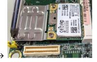
Step 3 There are two connectors on wireless LAN card. One is MAIN, and the other is auxiliary. Connect antenna cable to MAIN connector on wireless LAN card.
