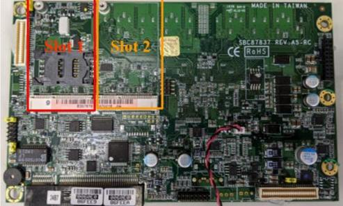
Step 1 Open the back cover and find out the mini-card slot on main board.
